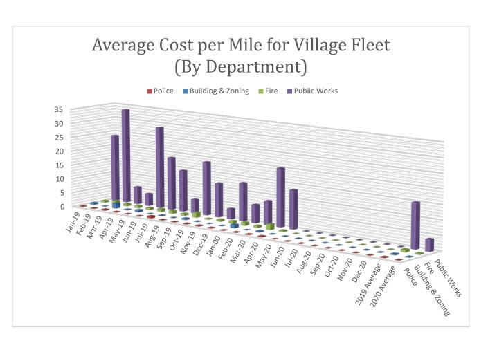
Vehicle cost per mile is an initial indicator of an efficient fleet operation. With basic cost per mile information in hand, all components that feed into that cost can be scrutinized and measured. These components include labor rates, fuel costs and parts costs. Looking further into the Village' vehicle cost per mile, staff can measure other components such as average vehicle age. When vehicles are replaced within their life cycle, the impact is usually positive.
